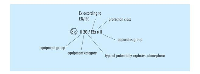
ATEX 95 has been implemented both in the EU member states and Switzerland. While approvals according to VGSEB (order on apparatus and protective systems for use in areas subjected to the risk of explosion) are restricted to Switzerland, electrical equipment for which a recognized monitoring body has issued a EU prototype test certificate with all required modules according to 94/9/EC can be introduced freely both in Switzerland and the European Union.
