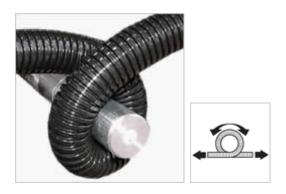
Cold bending test (DO 9.21-4380)
