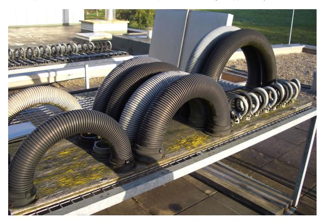
The other test specimens were also originally mounted on wooden boards but after more than 20 years of exposure to the elements the boards had deteriorated to such an extent that the product samples had to be remounted. The second time they were mounted on to a steel frame using clip.
