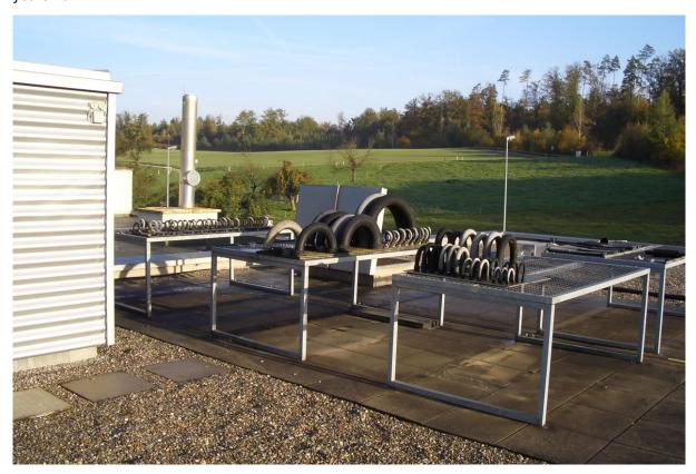
The following pictures show samples of various types of PMA polyamide conduit mounted on fixtures on the roof of the building. The deterioration of the wooden mounting plates themselves and the moss growing on them are an indication of the duration of exposure.
