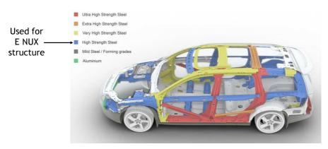
A comparison between the cabinet structure and the car structure can be made.
