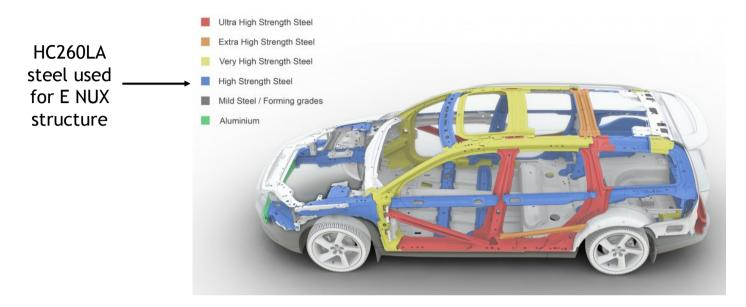
As a matter of fact, HC260LA sheet steel (EN10268) is included in the specifications of many car producers:
