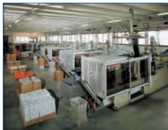
Moulding department for junction boxes in Pedrengo factory
