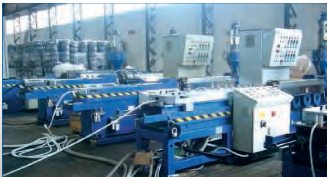
Extrusion department for pliable conduits in Osimo factory
