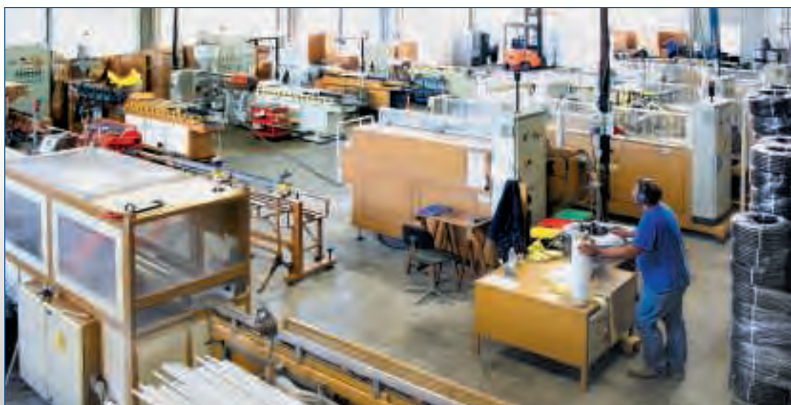
Extrusion department for rigid conduits in Avellino factory
