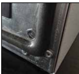
Polyurethane seal applied by continuous molding
