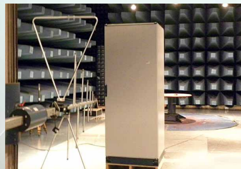
兩個接收天線——考慮頻率範圍。 Two receiving antennas in the frequency band considered.
